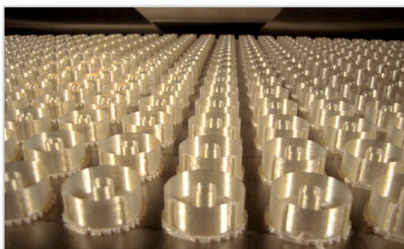
Kelly Manufacturing makes toroid housings using ULTEM 9085 on an additive manufacturing system. The method requires no tooling and offers the tight tolerance needed for this device.
